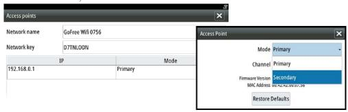
To set a device as secondary, the NSO evo2 must initially be connected to only one GoFree module. Pressing 'menu' with the device highlighted, opens the dialogue that allows setting to secondary. Once completed, a second module may be plugged in, and will automatically default to primary.
