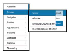
Devices with the Group set to None can be set to use different sources to those of the rest of the network devices.
