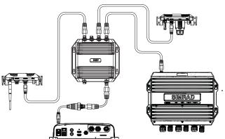
If the number of ethernet devices exceeds the number of available ports on the NEP-2, it is possible to link two or more NEP-2 modules together to provide the required ports. The NEP-2 modules are fitted with 5 ethernet ports.
